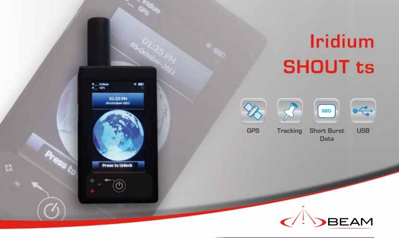
The **SHOUT** ts is a handheld, global, two-way satellite messaging and personal tracking device. It utilizes Iridium's short burst data (SBD) service to provide location information determined by a GPS receiver, two-way inbound and outbound status, text messaging, and emergency/alert notifications.
